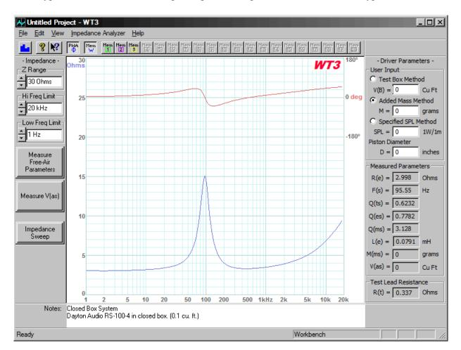
Here is a typical result when measuring a single full range driver in a closed box type enclosure:
